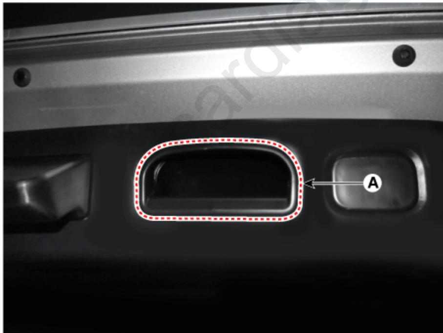
4. Separate the smart tailgate inner switch (A).
